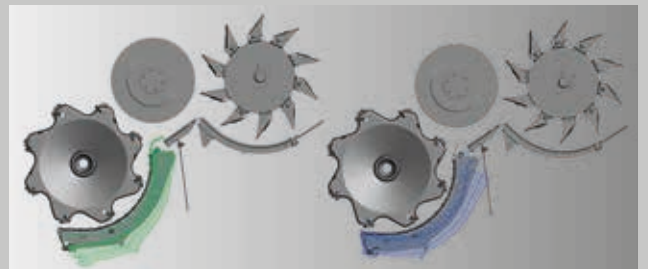
Concave adjustment independently in the front and rear.
