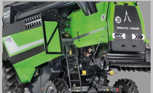
Easy access to the upper part of the combine as well as to refill Diesel.
