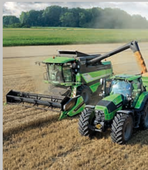
Unloading tube to discharge the grain while working in any position to tall trailer.
