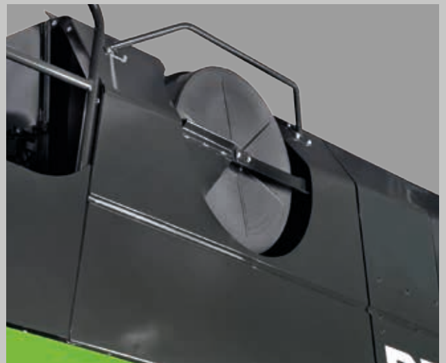
Big rotary screen to ensure maximum efficiency of the cooling system.
