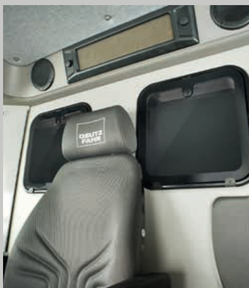
Double grain tank inspection window.
