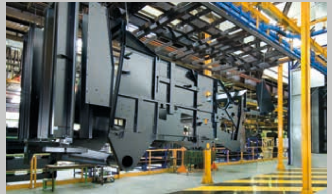
All components treated with cathoresis and automotive painting process.
