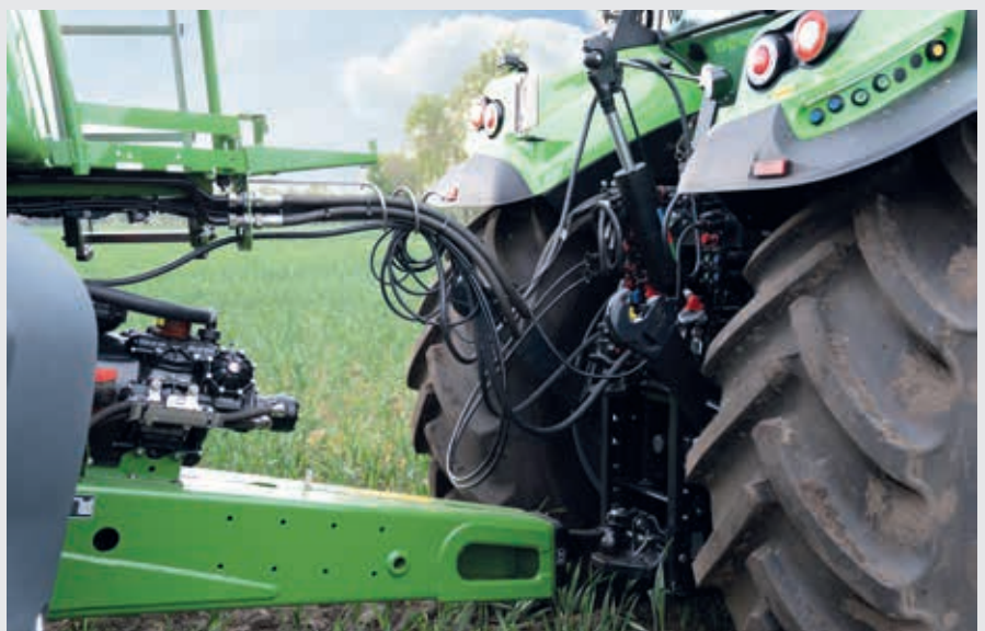
↑ Rear linkage in transport position for less interference with drawbars while cornering.
