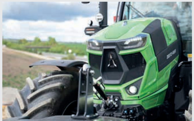
↑ LED driving lights and characteristic LED worklights.
