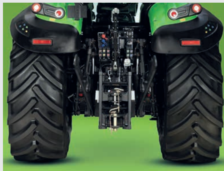
Rear linkage, five rear spool valves, external controls on fenders on both sides.
